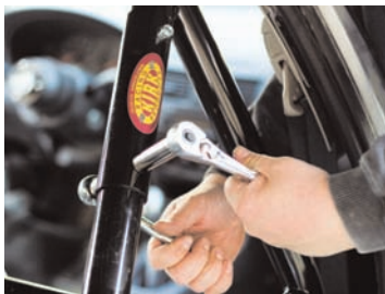
(ABOVE) Recycling items like the seat and harness from another project helped us save money. (LEFT) The Kirk Racing Products bolt-in roll cage fit perfectly and installed with simple hand tools. (BOTTOM LEFT) When using a bolt-in roll cage, take special care to follow the manufacturer's instructions, double checking the GCR that the cage will be legal.
