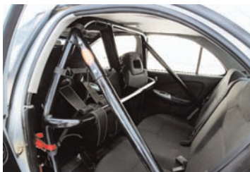
(ABOVE) Recycling items like the seat and harness from another project helped us save money. (LEFT) The Kirk Racing Products bolt-in roll cage fit perfectly and installed with simple hand tools. (BOTTOM LEFT) When using a bolt-in roll cage, take special care to follow the manufacturer's instructions, double checking the GCR that the cage will be legal.
