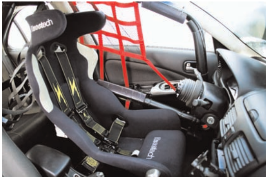
(ABOVE) Recycling items like the seat and harness from another project helped us save money. (LEFT) The Kirk Racing Products bolt-in roll cage fit perfectly and installed with simple hand tools. (BOTTOM LEFT) When using a bolt-in roll cage, take special care to follow the manufacturer's instructions, double checking the GCR that the cage will be legal.
